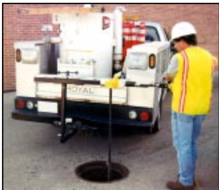
Pow-R-Arm supports the valve operator, swivels 180°, telescopes 18" and quickly mounts to vehicle trailer hitch.
